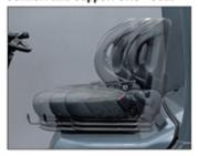
The ORS seat can be adjusted 150 mm forward and backward to provide comfort and support to almost all sizes of operators. \*ORS: Operator Restraint System
