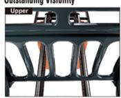
The overhead guard, mast and instrument panel have been designed to provide excellent visibility of the fork tips at the most frequently used lift heights.
